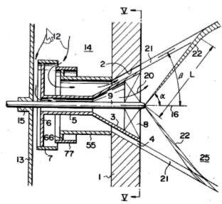
2. Liquid fuel is entrained into the combustion space by a stream of gaseous medium, for example, air or steam
