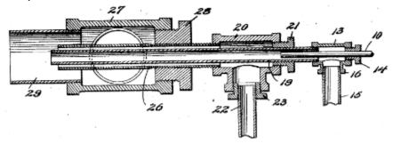
3. Liquid fuel is vaporised within a conduit and released in gaseous form into the combustion space
