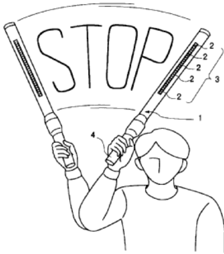
Figure 6 illustrates a baton using light emitting cell array to form a display.
