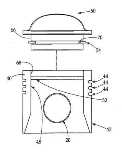
The Figure illustrates a multi-part piston assembly comprising a piston head (60) having a cylindrical member (66) that is inserted into an upper cylindrical opening (68) of a piston body (40) and secured via a locking ring (54) to the piston body (40).
