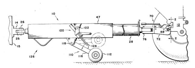
2. Bars connectable to an aircraft for manually turning or towing:
