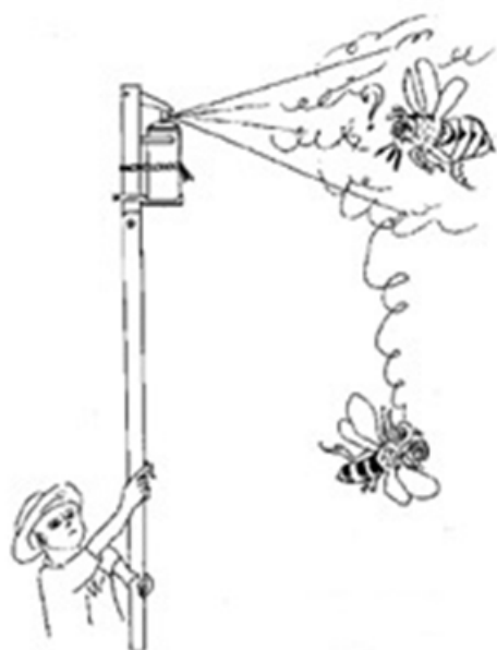
Figure 1 illustrates a pole for use in supporting an aerosol spray container used to exterminate insects, e.g wasps.
