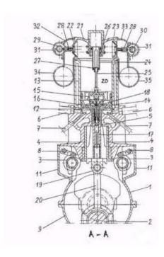
Engine with pulled con-rods during working stroke.
