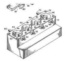
{Comb filters or interdigital filters with metallised resonator holes in a dielectric block}
