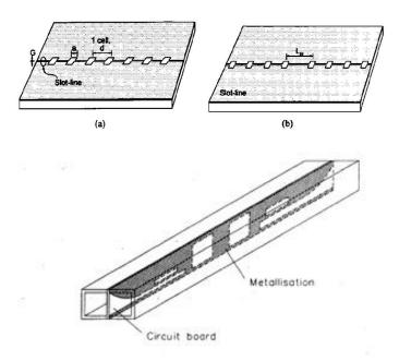
Figure 1. The new E-plane filter.
