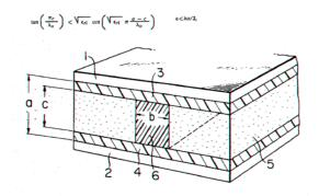
In this figure, 1 and 2 are metal layers, 3 and 4, dielectric layers and 6 is a low loss high dielectric constant dielectric.
