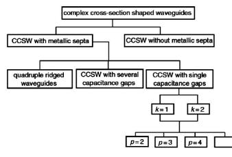
Fig. 1 Classification scheme of waveguides with complex cross-sections
