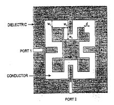
The microstrip loop resonator B includes an open conductive loop with folded transmission line segments extending from the adjacent ends of the loop formed on dielectric substrate.
