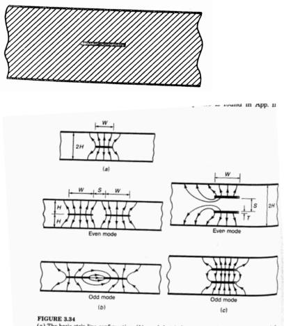
(a) The basic strip-line configuration; (b) coupled strip line using coplanar strips; (c) coupled strip line using broadside coupled strips. The electric field lines for the TEM modes are also shown.
