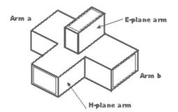
Magic T waveguide junction
