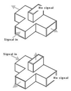
Magic T waveguide junction signal directions
