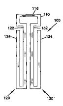
The hairpin resonator disposes a substrate of finite thickness is embedded inside a shielding box and is used as support for the metallized plane.
