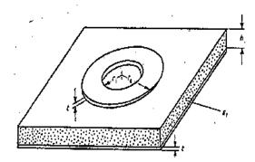
A rectangular micostrip disk can be considered as a degenerated microstrip line having line-width w and line-area  $\pi^* \text{ro2}$
