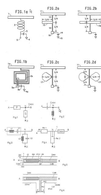
Filters for transverse electromagnetic waves (<u>H01P 1/212</u>, <u>H01P 1/213</u>, <u>H01P 1/215</u>, <u>H01P 1/219</u> take precedence)
