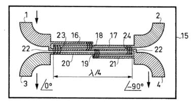
Lange couplers are generally used to couple electromagnetic energy between transmission lines. In a four port hybrid, there is an input port and a direct port, these two ports being directly and conductively connected to each other, as well as a coupled port, the latter being connected to transmission lines coupled electromagnetically (inductively and capacitively) to the conductors extending between the input and direct ports.
