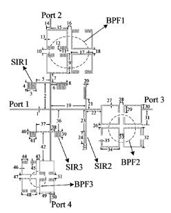
Fig. 5. Layout of the proposed microstrip triplexer.
