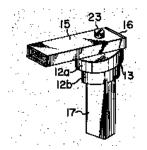
{the energy being transmitted in at least one ring-shaped transmission line located around the axis of rotation, e.g. "around the mast" rotary joint (H01P 1/069 takes precedence; coaxial line with solid inner conductor H01P 1/067)}
