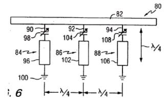
Bandpass filters using ring resonators with different notch frequencies connected in parallel (see US2007/0063794).
