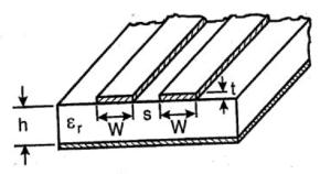
Figure 3.20 Edge-coupled microstrip lines.
