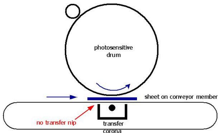
**G03G 15/1665****{by introducing the second base in the nip formed by the recording member and at least one transfer member, e.g. in combination with bias or heat}****Definition statement***This place covers:*
