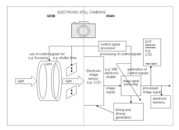
In the above image, elements on the left side correspond to <u>G03B</u> (e.g. light, use of control signals for focusing and shutter time). Elements on the right side correspond to <u>H04N</u> (e.g. control signal
