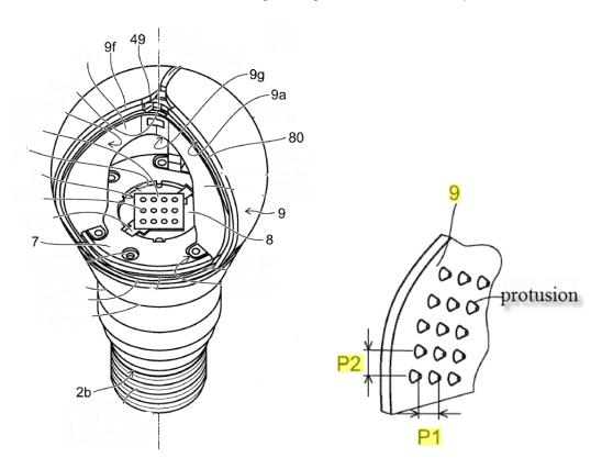
Globe forming fins or the exterior of which in contact with fins. See illustrative example below:
