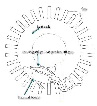
Heat insulating material between components to prevent heat conduction in figure below:
