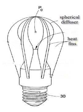
Evaporation and condensation within the globe of the lighting device or LED module or LED lamp, i.e. part of a globe is forming a part of a heat pipe. See illustrative example below:
