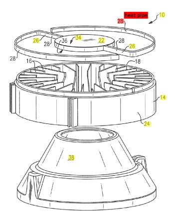
Evaporation and condensation within the globe of the lighting device or LED module:
