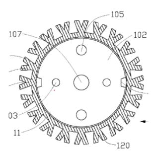
{the planes containing the fins or blades having directions perpendicular to the light emitting axis}
