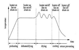
The above diagram represents a typical drying method for laundry dryers, belonging to D06F 58/30 in which, during the drying process, the heater and the blower fan are subsequently turned ON/ OFF while the drum is rotated. It is noted that D06F 58/30 relates to methods for treating the laundry
