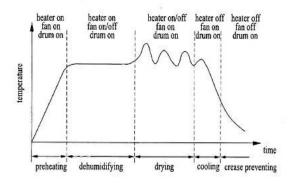
The above diagram represents a typical drying method for laundry dryers, in which several laundry treating steps are performed, for example during the drying process the heater and the blower fan are subsequently turned ON/OFF while the drum is rotated.
