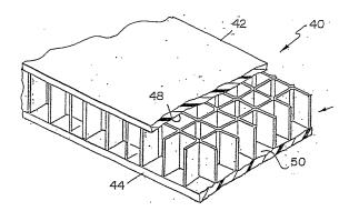
characterised by a face layer formed of separate pieces of material {which are juxtaposed side-by-side (B32B 5/02 takes precedence)}
