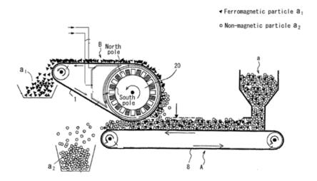
This example shows a combination of magnetic separating belts with material carrying belts in which a material carrying belt (8) is working in conjunction with another belt (1) that is magnetized by a magnetic roll (20).
