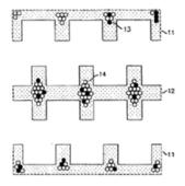
This example shows an electrode arrangement comprising interdigitated electrodes (11) and (12) that create an open-gradient electrostatic field.
