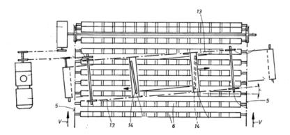
This example shows multiple belt carriers characterised by their mutual disposition in which magnetic bars (6) are moved by endless conveyor chains (5) and a set of conveyor chains (13) having drive scrapers (14) at an oblique angle with respect to the magnetic bars (6).
