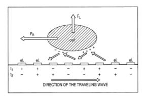
This example shows an electrode arrangement to which a time-varying electric field is applied for movement of a biological cell when polarised by the electric field.
