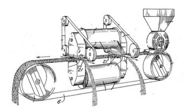
This example shows a cross belt magnetic separator having a main conveyor belt (6) and cross belts (21).
