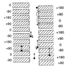
This example shows the response of particles exposed to a travelling wave field with a phase shift in between neighbouring electrodes.
