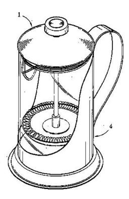
Example of a coffee machine of the type "French press" (from US6186052 by Huang)
